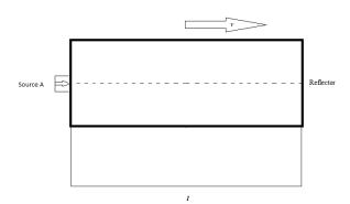
Single clock is used to avoid errors due to synchronization between different clocks at different locations. A laser source and a clock are placed at A similar to above methods. A perfect reflector is placed perpendicular to the direction of motion which helps to return the light ray.
